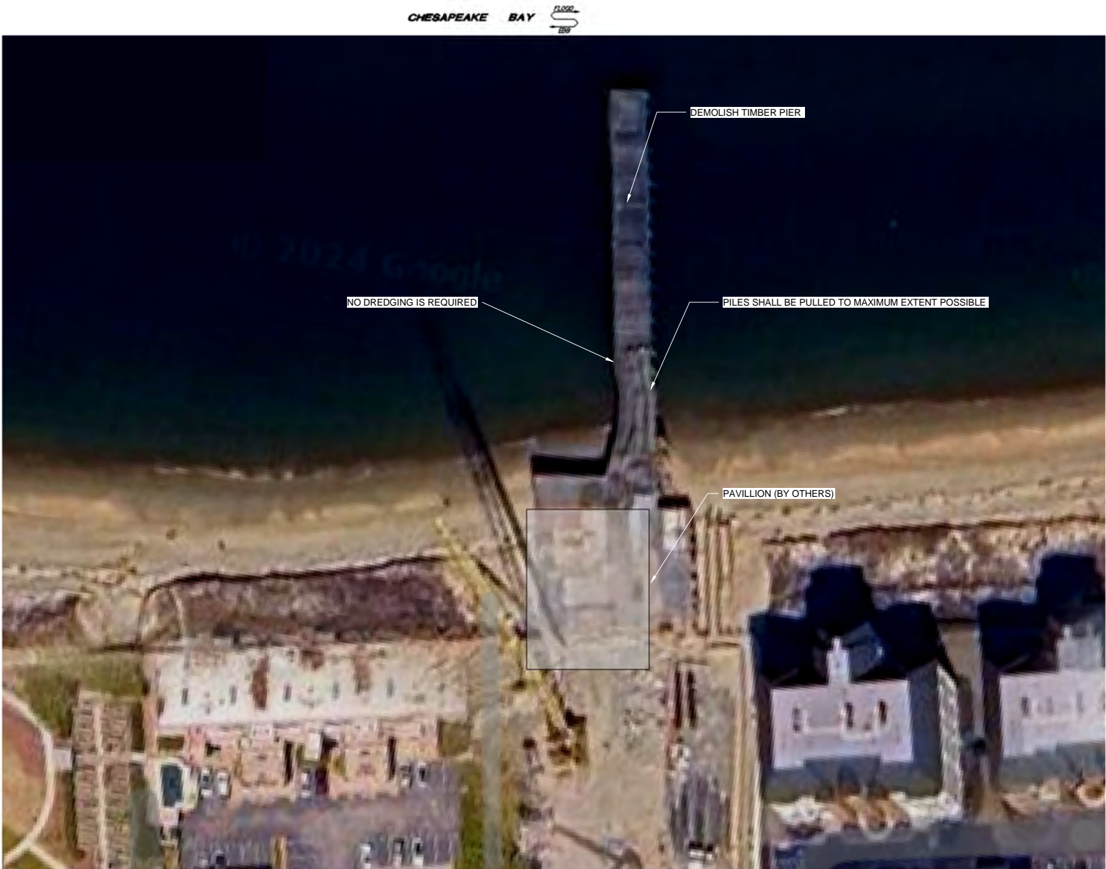
PIER DEMO PLAN 1 SCALE: 1" = 10'-0"
